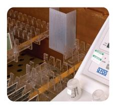
To conduct accelerated corrosion testing in the laboratory, a Q-Fog machine exposes panels to a cyclic environment of salt-laden fog, heat, and humidity.
